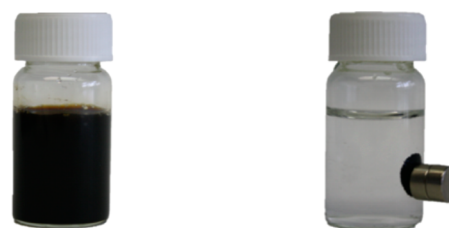
Figure 3. Fe 3 O 4 (TMS-EDTA) nanoparticles dispersed in water (left) and the retrieval using a permanent magnet (right).
